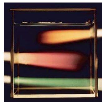
Figure 12.15 Three beams of white light, passing through a colloid of sulfur particles in water, change to orange, pink, and bluish-green. The colors produced depend on the size of the particles and also on the position of the viewer. The smaller the dispersed particles, the shorter (and bluer) the wavelengths.
