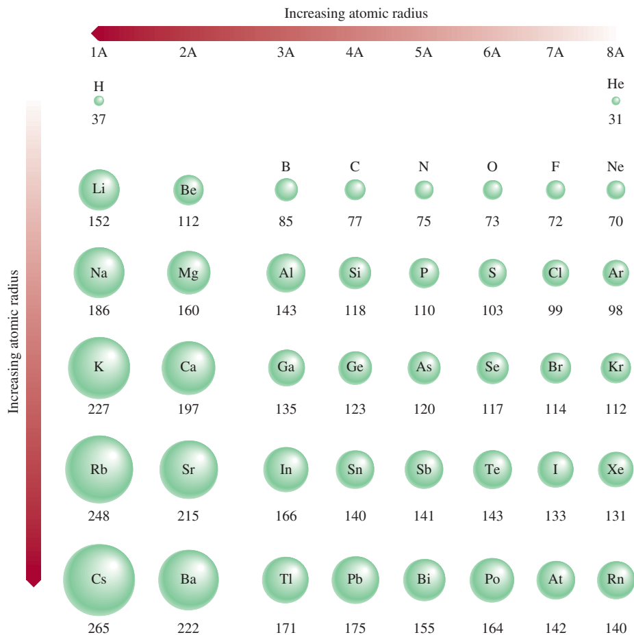
Figure 8.5 Atomic radii (in picometers) of representative elements according to their positions in the periodic table. Note that there is no general agreement on the size of atomic radii. We focus only on the trends in atomic radii, not on their precise values.
