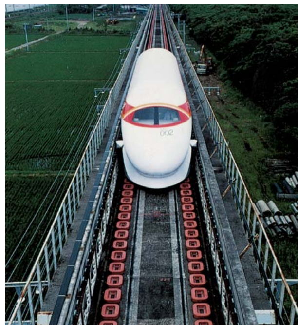
An experimental levitation train that operates on superconducting material at temperature of liquid helium.
