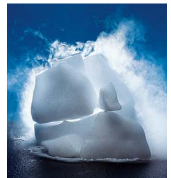
Figure 11.42 Under atmospheric conditions, solid carbon dioxide does not melt; it can only sublime. The cold carbon dioxide gas causes nearby water vapor to condense and form a fog.
