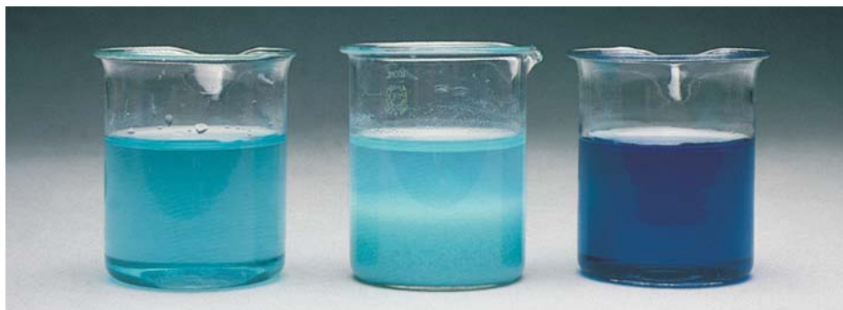
Figure 16.11 Left: An aqueous solution of copper(II) sulfate. Center: After the addition of a few drops of a concentrated aqueous ammonia solution, a light-blue precipitate of \text{Cu}(\text{OH})_2 is formed. Right: When more concentrated aqueous ammonia solution is added, the \text{Cu}(\text{OH})_2 precipitate dissolves to form the dark-blue complex ion \text{Cu}(\text{NH}_3)_4^{2+} .
