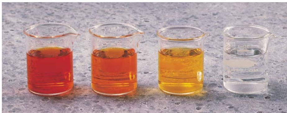
Figure 13.3 From left to right: The decrease in bromine concentration as time elapses shows up as a loss of color (from left to right).
