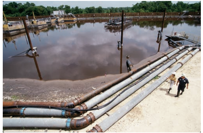
A Superfund site in Houston, Texas, where bacteria were used to clean up harmful industrial waste.
